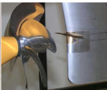
Slika 36. HHI Thrust Fins (ABS)
