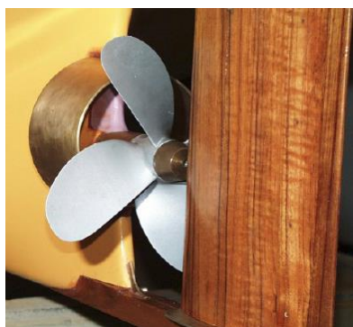
Slika 40. Integrated Lammeren Duct, ABS
