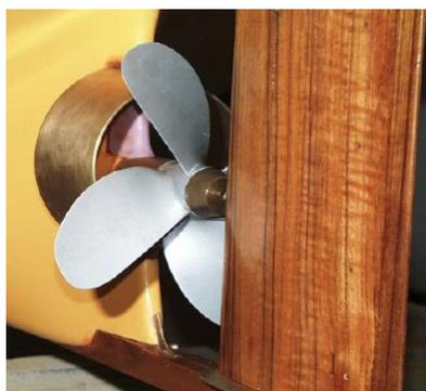
Slika 40. Integrated Lammeren Duct, ABS
