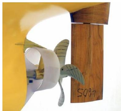
Slika 41. ModelBMS Mewis Duct®- ABS
