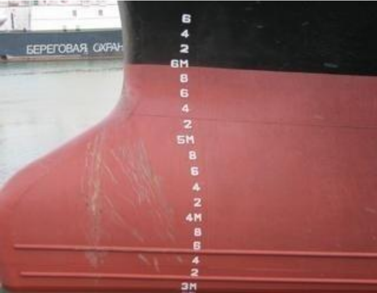
Figure 3. Hull of boat marked with draught depth (source: http://balticcontrol.ru/wp-content/gallery/draft-survey/img_3647.jpg )
