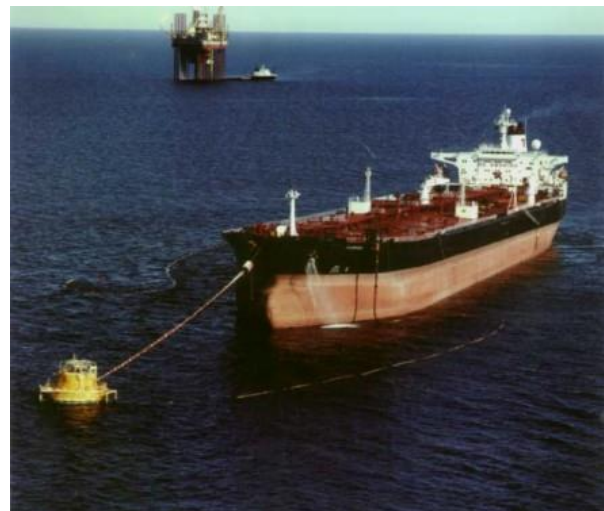
Picture 15. Single buoy mooring
