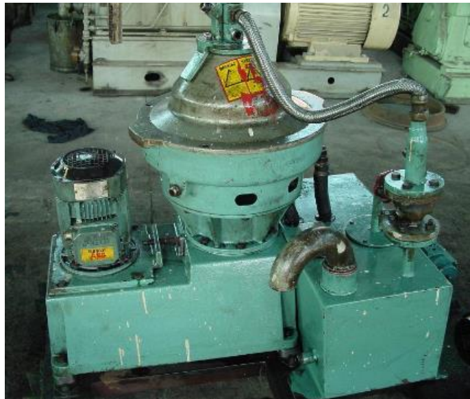
Slika 8. Brodski separator, (Izvor: Internetska stranica Exspters India , rifuge-2256 https://www.exportersindia.com/product-detail/alfa-laval-centrifuge-mmpx-303-sgp-11-60-oil-purifier-separator-cent96.htm )
