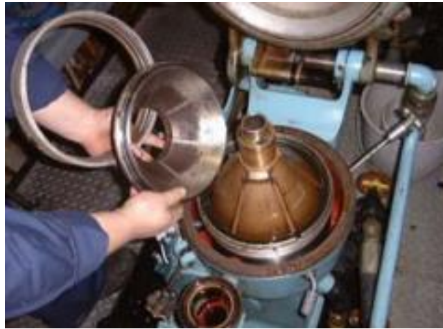
Slika 12. Gravitacijski disk (Izvor: The Alfa Laval MAB separator, Tehnical notes of interest to Marine Engineers)
