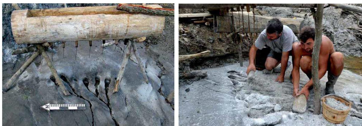
Fig. 7 Rock salt piercing using a wooden trough and consequent extraction of rock salt in Băile Figa near Beclean, northern Transylvania, Romania (Buzea 2018: 69, 111).
