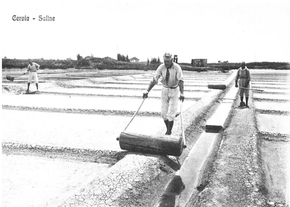
Fig. 31 Cotice ("cotg") employed in the salt pans of Cervia at the beginning of the 20th century (courtesy of Nino Giunchi).
