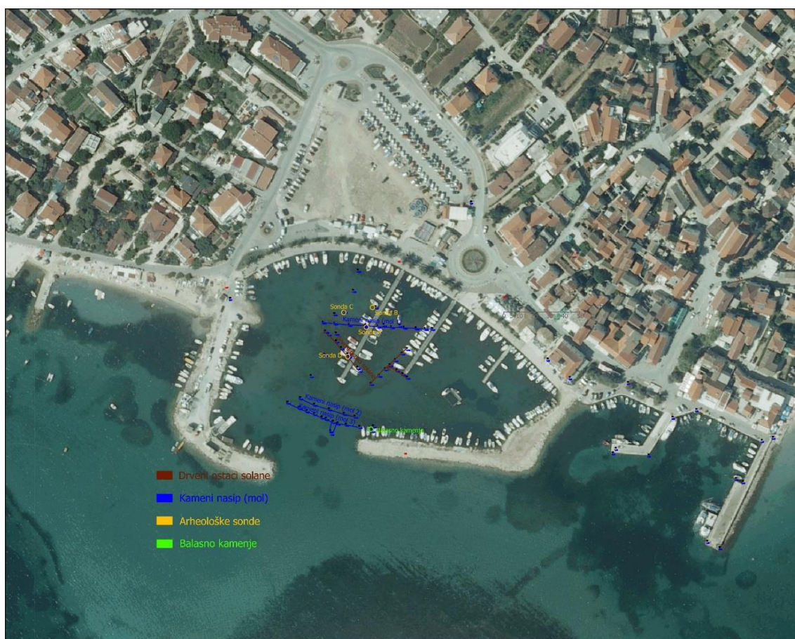
Fig. 212 Structures recorded in 2005: blue = stone embankments, brown = wooden remains of the probable saltpan, yellow = archaeological probes, green = ballast stones (K. Zubčić, from Radić Rossi et al. 2018, fig. 9).
