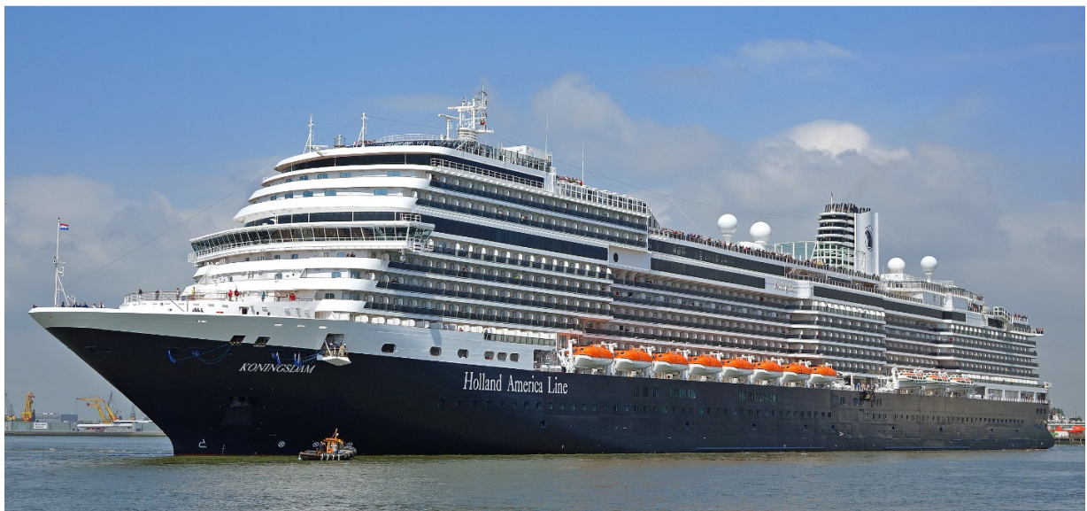
Slika 11. M/V Koningsdam, (Loa = 297 m, B = 35 m)
