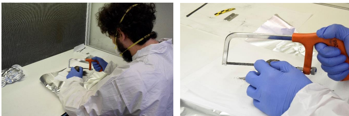
Fig. 9-17. and Fig. 9-18. Cutting lead white ingots at the Department for Geochemistry, Vrije University, Amsterdam, Netherlands (photo: K. Batur).
