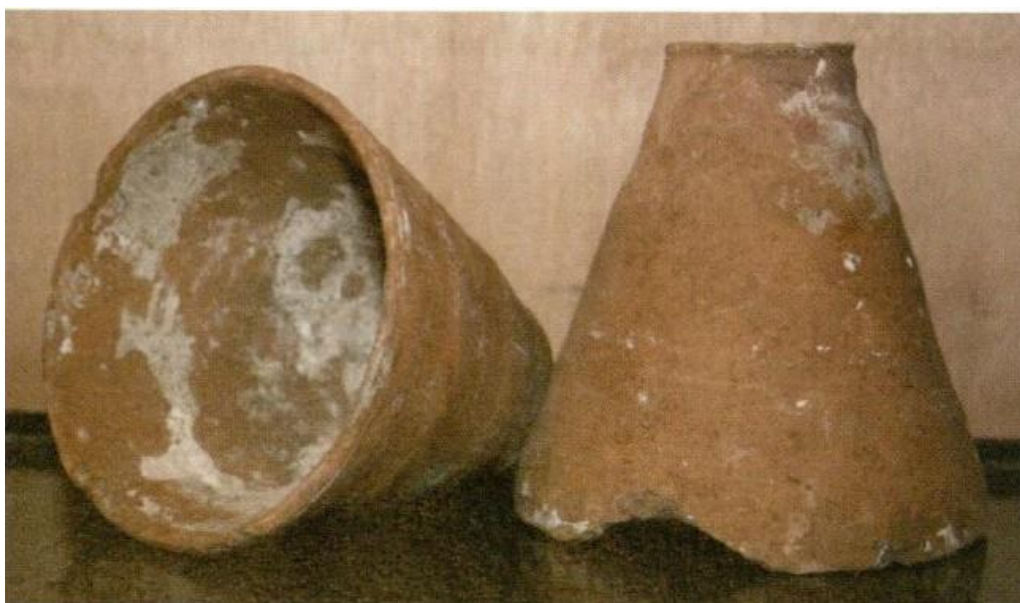
Fig. 9-19. Lead white was manufactured in conical ceramic moulds. This example represents the lead white mould from the mill ‘De Rob’, Koog an de Zaan, Netherlands, collection of Mollenmuseum (Stols-Witlox 2011, p. 288).
