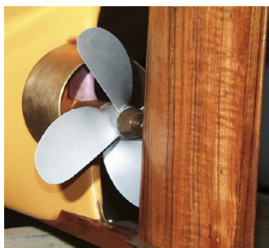
Slika 40. Integrated Lammeren Duct, ABS
