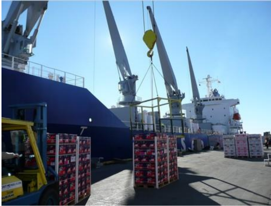
Picture 7. Loading palletized cargo
