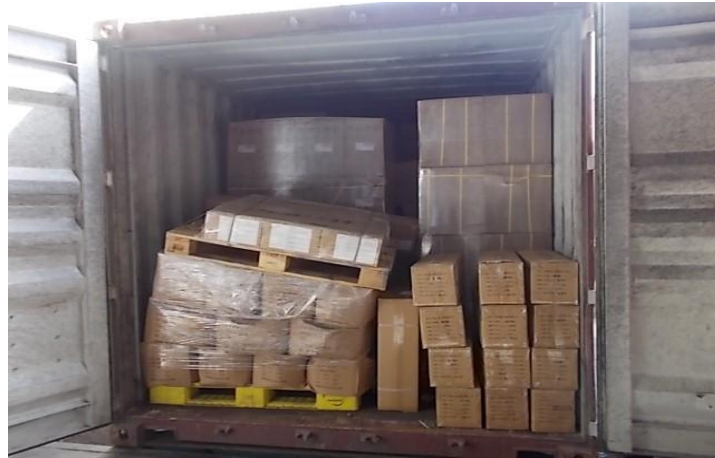
Picture 4. Poor cargo securing
