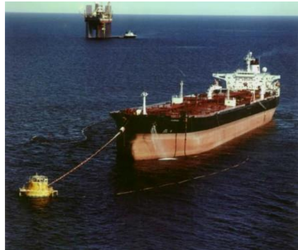
Picture 15. Single buoy mooring
