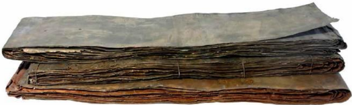
Fig. 9-53. Brass processed and stacked into sheets ( Bugmessing ). Average length is 73 cm, and width 18 cm (Cassitti 2018, p. 49)
