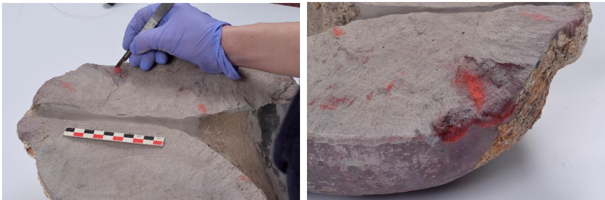
Fig. 9-27. and Fig. 9-28. Grey alteration layer of bell-shaped mercury sulphide, type A (photo: N. Čuk).
