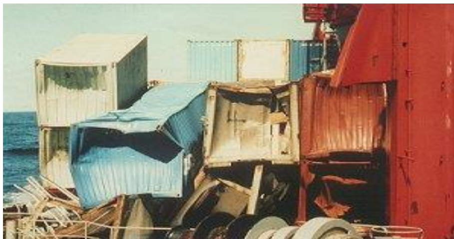
Picture 5. Cargo damaged by breaking wave impact
