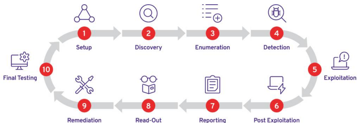
Slika 11 Proces penetration testinga, Izvor: https://plextrac.com/blog/hack-the-10-steps-of-the-pentesting-routine/
