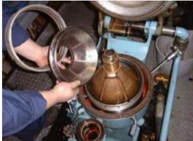
Slika 12. Gravitacijski disk (Izvor: The Alfa Laval MAB separator, Technical notes of interest to Marine Engineers)
