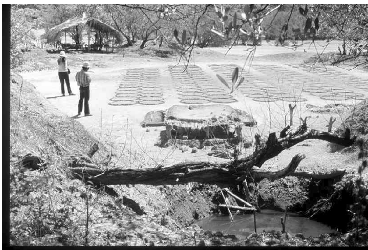
Fig. 45 Salt making in Chacahua, western Mexico: the well (foreground), the filtering device, round solar evaporation salt pools and mounds of leached earth (at the sides) (photo of David Grove, from Williams 2015).
