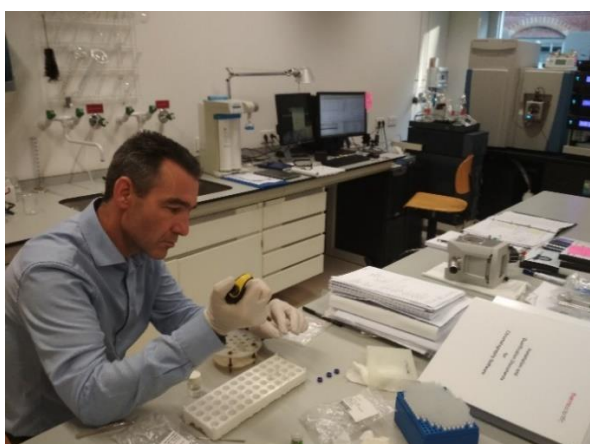
Fig. 4-23. and Fig. 4-24. M. van Bommel performing UHPLC analyses on the samples of Gnalčić lake pigment in Ateliergebouw, Amsterdam. Instrument: Waters Chromatography Acquity H-Class (photo: K. Batur).
