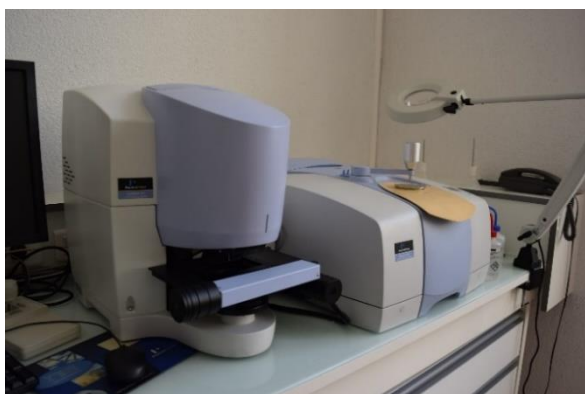
Fig. 4-21. FTIR instrument: Imaging System, Perkin Elmer (photo: K. Batur).
